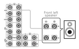
Since both front and surround back speaker terminals output the same audio, it doesn't matter which set (front or surround back) is powering which part (**Hi** or **Low**) of the speaker.
